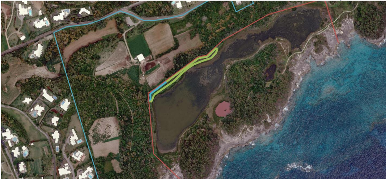
Figure 16 The area marked in aqua shows the length and location of the proposed ditch and berm. The area marked in green shows the area to be planted in native and endemic flora. It should be noted that some of the work will take place on the Government of Bermuda owned part of the Nature reserve. Permission has been provided by the appropriate minister and the Department of the Environment and Natural Resources (see letter inclusive of a map provided).
